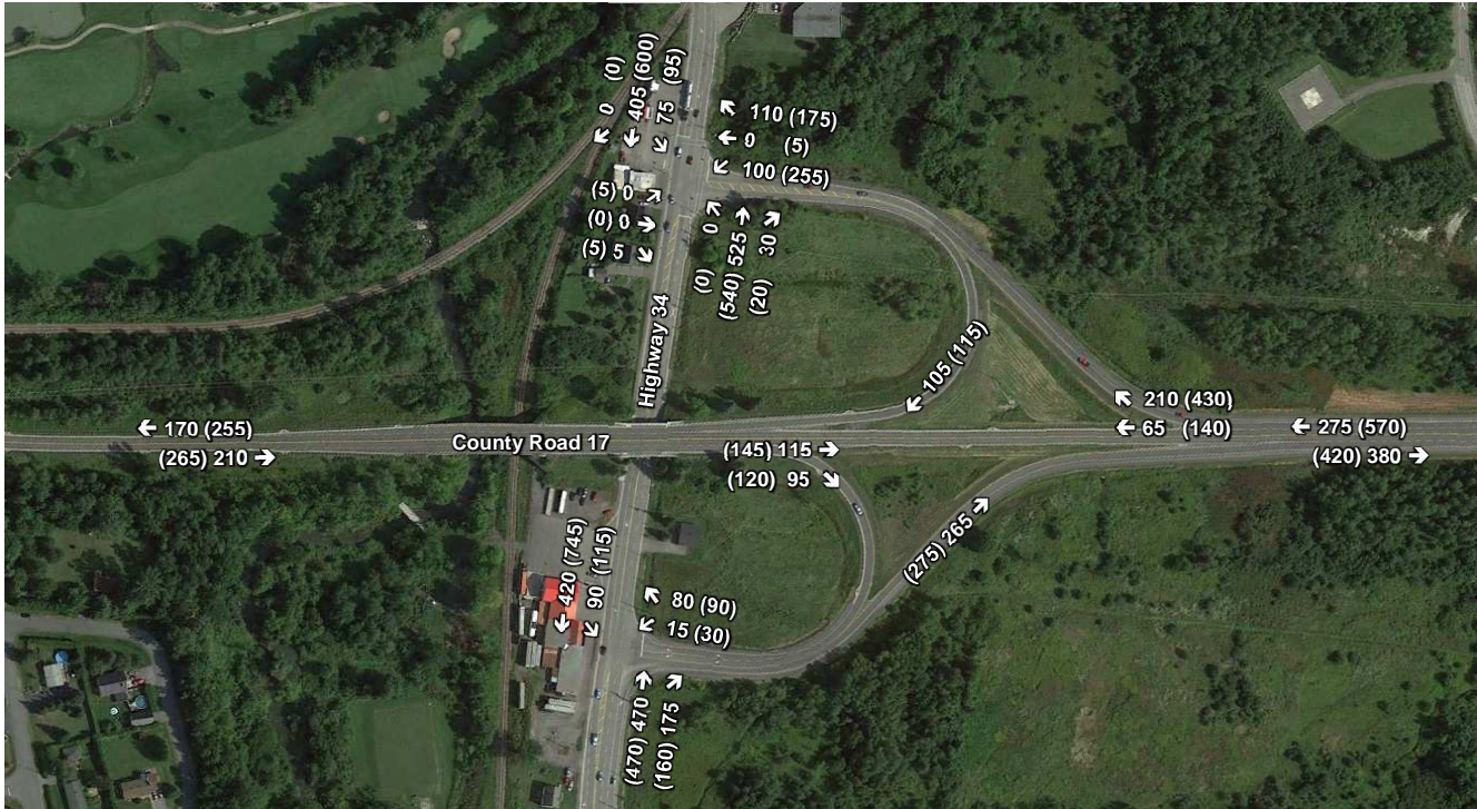
Figure 1: Existing Interchange Configuration and Traffic Volumes
